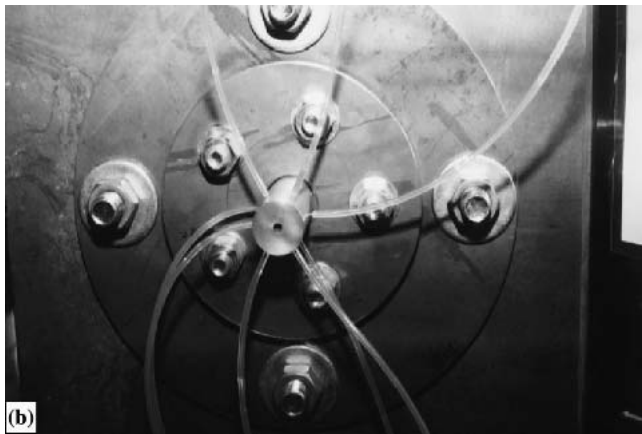
Fig. 11 (a) Cold gas dynamic spray gun system, not to scale; (b) photograph of the nozzle and pressure lines
